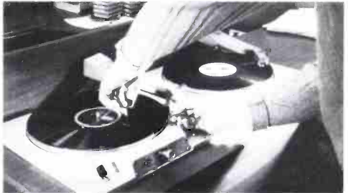
Using a device such as the Watts Disc Preener is probably the quickest and most effective way to add 10 dB to the dynamic range. It should be included as a part of the record cuing process.
