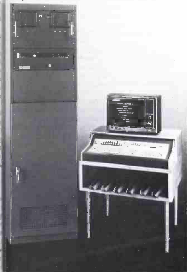
Chiron Graphics II system has, like Vidifont, digital storage of variety font styles, can reproduce logos, symbols, almost any graphic material. Long-term message storage is on "floppy discs," which hold up to 2000 lines of characters at one time.
