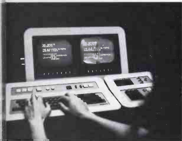
CBS Vidifont system has two screens, one on which message can be assembled, the other to monitor video with message coded. Standard typewriter keyboard allows message to be entered; as on most character generators, message is held in memory until needed.
