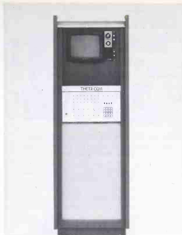
Theta-Com Series 100 systems can take information from news, weather, and financial wire systems, and from local and remote-access keyboards. The remote keyboards can be used by public officials, educators, advertisers to put messages directly onto "local" cable channels.
